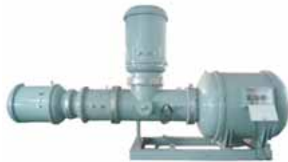
800kVA/800kV testing system (with encapsulated coupling capacitor, HV measurement capacitor, PD standard injection port and connection flange)
